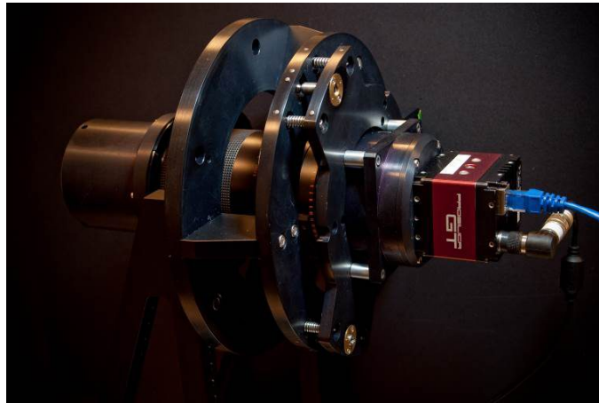
Figure 7. Metrology system camera assembly for TAIPAN.
